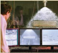
and top/bottom flow split, the BETE DTH provides a significant performance and cost advantage. With flexibility in the design, many applications require no piping modifications, making the BETE DTH ideal for the scrubber retrofit market. Of course, all DTHs are made with Silicon Nitride Bonded Silicon carbide, guaranteeing a service life of ten years or more.\*
