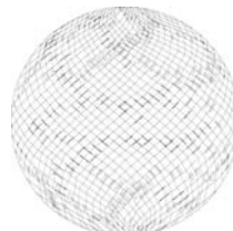
Orbitor 4 nozzle spray pattern
