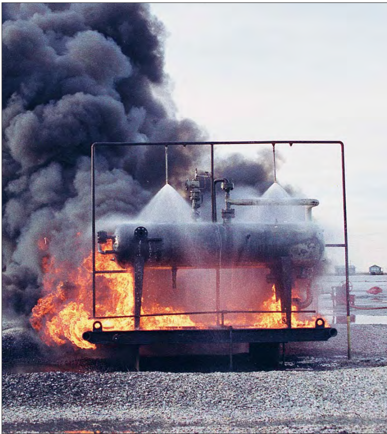
N6 nozzles protect a propane storage tank from fire and explosion.
