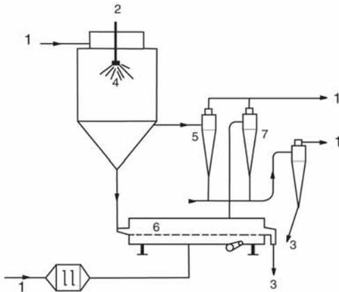
**Two Stage Dryer with Vibrating Bed Dryer**
