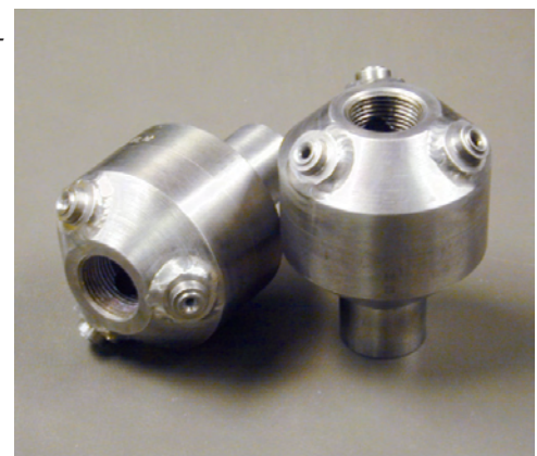
CLUMP, cast and welded in Tantalum
