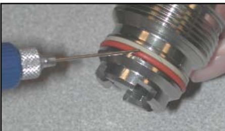
Apply lube to the o-ring on the body before installing into the carrier (We do not want the o-ring to stick to the carrier when it is being threaded on).
