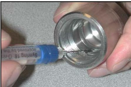
Use lubricant supplied by BETE or equivalent (i.e.: Lubri-film or Superlube) to coat the inside of the carrier where the o-ring seats. Make sure there are no dry areas.
