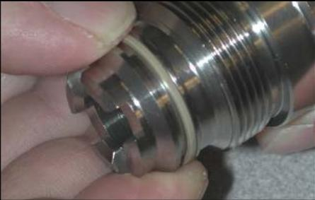
**This step is only for the high pressure Twist & Dry (TD-K) nozzle.** Install the backup ring into the body o-ring groove. The backup ring has a split bias cut which allows it to expand to fit over the body o-ring groove. Once the backup ring is over the body o-ring groove, it can be released and it will snap into place. Make sure the backup ring is positioned in the o-ring groove and pushed toward the inlet connection end of the body.
