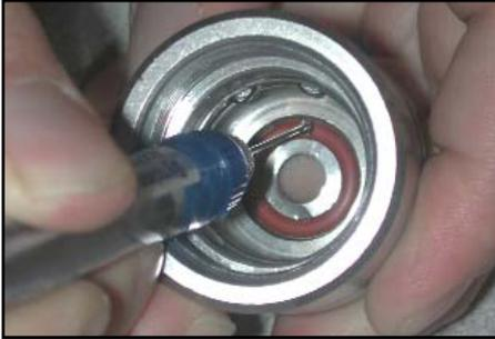
Apply lube to the installed orifice o-ring.
