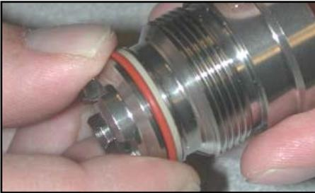
**This step is only for the high pressure Twist & Dry (TD-K) nozzle.** Make sure the o-ring is positioned in the groove, next to the backup ring and away from the connection end of the body.
