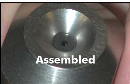
The carrier need only be **HAND TIGHTENED, DO NOT WRENCH TIGHTEN!** Check to see that the orifice is seated against the inside of the carrier.
