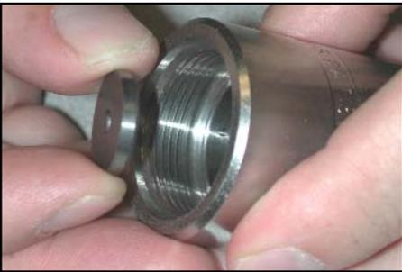
Put the selected orifice disc on top of the o-ring, with beveled outside edge facing o-ring.
