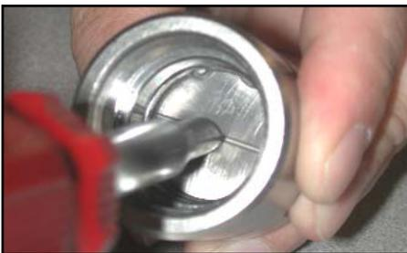
Using a screwdriver, turn the swirl 1/4 turn so that it is secured into place under the 2 lugs. (No turning is necessary for lugless carriers)
