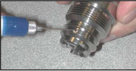
Apply lube to the body threads and o-ring groove generously. Lubricant needs to be in the o-ring groove so the o-ring will not stick to the body when the carrier is tightened down or removed.
