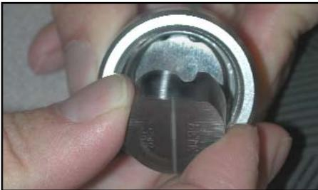
Install the swirl into the carrier, swirl side toward orifice disc. (TIP: hold the carrier at a 45 degree angle with the 2 lugs at 12 o'clock. Align the flat side of the swirl at 12 o'clock. The swirl will drop into place).
